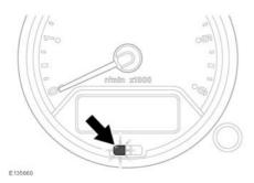
The alarm status is displayed by the indicator. After locking the vehicle, one of the following will be indicated.
