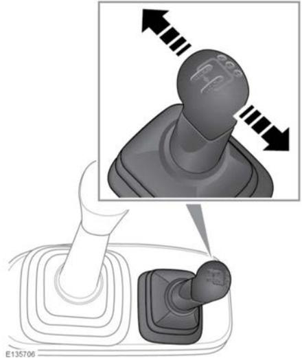
**High range:** Use for all normal road driving and when off-road driving across dry, level terrain.
