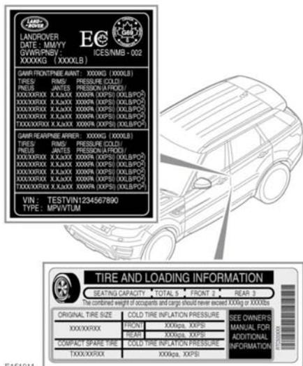
The recommended tire pressures are listed on a label located in the driver's door opening.
