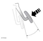
The brake pedal travel is set at the factory and is non-adjustable. The brake pedal free travel is up to 5 mm.
