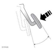
The brake pedal travel is set at the factory and is non-adjustable. The brake pedal free travel is up to 5 mm.
