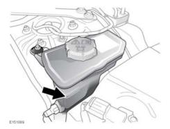
The fluid level should be maintained between the **MIN** and **MAX** marks.
