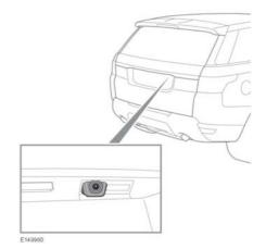
When Reverse  $(\mathbf{R})$  is selected, the screen automatically displays a wide-angle, colour image from the rear of the vehicle.
