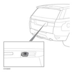
When Reverse (R) is selected, the screen automatically displays a wide-angle, colour image from the rear of the vehicle.
