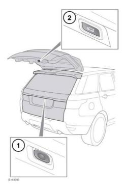
1. Tailgate open/close using the exterior button. Press to open, stop, reverse direction or close the tailgate.
