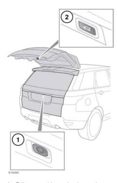
Tailgate open/close using the exterior button. Press to open, stop, reverse direction or close the tailgate.
