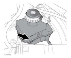
The driver's side cover must be removed to check the brake fluid level. See 210, UNDER BONNET COVERS - REMOVAL.
