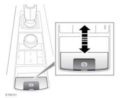
With the ignition turned on, press the brake pedal and press down on the EPB switch. This will release the EPB.
