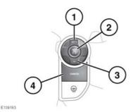
SET+: Press to set the speed or to increase the set speed. The cruise control indicator illuminate to confirm cruise control is operational (see 53, CRUISE CONTROL (GREEN)).
