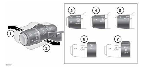
With the headlamps on, push the control away from the steering wheel to select high beam. The warning lamp will illuminate. See 53, HIGH BEAM (BLUE).
