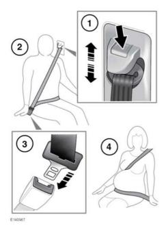
Seat belt height adjustment: Press to release the catch.
