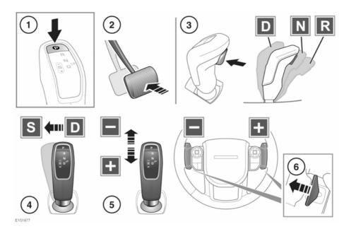
The gear selector status is displayed in the Message centre. See **46**, **INSTRUMENT PANEL**. Also the appropriate LED indicator, on top of the gear selector, will illuminate to confirm selection.
