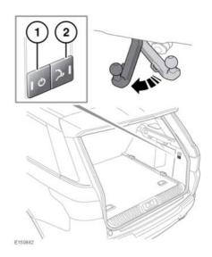
The powered tow bar is hidden in its stowed position behind the bumper. It can be deployed using the buttons located on the right side of the loadspace.
