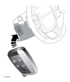
Position the Smart key flat against the side of the steering column with the buttons facing outwards.
