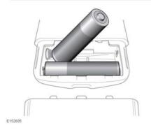
Low battery power is indicated by the remote control power button flashing 3 times when pressed. To renew the batteries:
