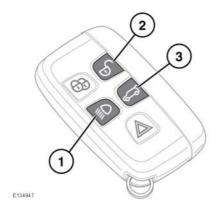
To raise the vehicle press and hold button (1) and button (2) together.
