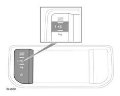
A short press of the Park assist button will turn the system on. When Park assist is switched on, the button LED will illuminate. The Park assist button can be used to scroll through the 3 Park assist features:
