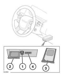
To install a SIM card, press the button (1) to release the SIM card holder (2). Insert the SIM card into the holder as indicated (3).
