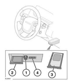
To install a SIM card, press the button (1) to release the SIM card holder (2). Insert the SIM card into the holder as indicated (3).
