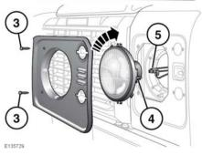
In order to change a headlamp unit bulb, you must first remove the headlamp unit:
