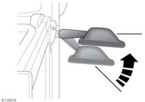
The mirrors are designed to fold to the side on impact. They can also be folded when negotiating narrow gaps.
