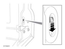
Child safety locks are fitted to the rear doors to allow you to prevent accidental opening of the doors when the vehicle is in motion. If children are to be carried in the rear seat positions, it is recommended that the child safety locks are used.
