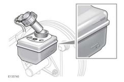
Inspect the fluid level through the side of the transparent reservoir. The fluid level should be between the **MIN** and **MAX** marks.
