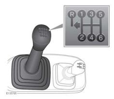
The transmission consists of a 6 speed manual gearbox and a high/low range transfer box. A centre differential distributes the drive to the front and rear axles, providing permanent four wheel drive.
