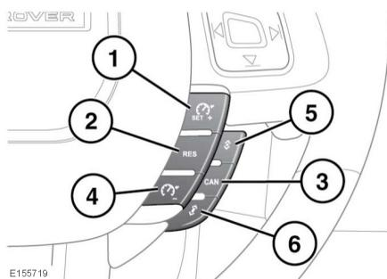
1. Press to set the vehicle's current speed as the set speed. The ACC warning lamp will illuminate to confirm ACC is operational. See **46, CRUISE CONTROL (GREEN)**. While ACC is enabled, further pressing of the button will raise the set speed above the vehicle's current speed. The speed of the vehicle will gradually increase to reach the new set speed.
