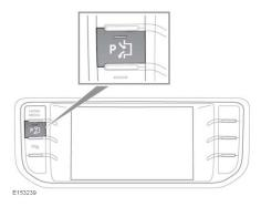
A short press of the Park assist button will switch on the Park assist system. Further presses will scroll through the Park assist options. To switch off the system, repeatedly press until the LED on the button extinguishes.
