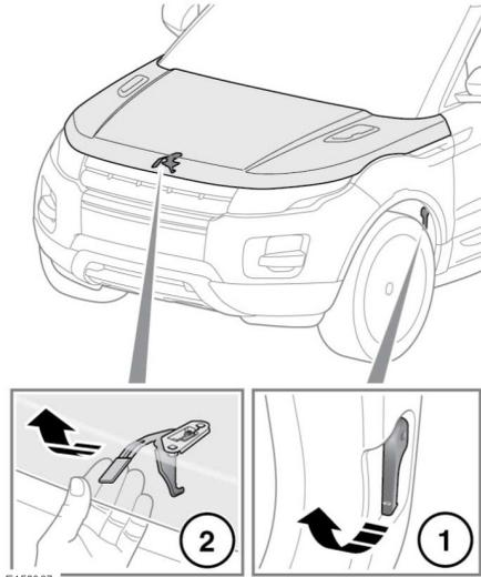
1. Pull the bonnet release lever, located in the left side front footwell.
