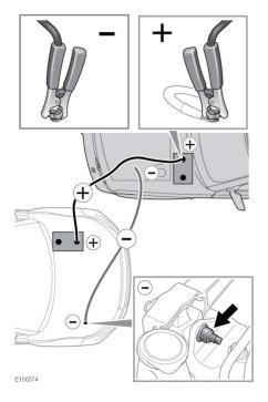
Connect the positive (Red) jump lead to the recommended positive (+) boost terminal on the donor vehicle.
