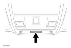
An airbag status indicator lamp, mounted on the overhead control panel (as illustrated), will display the operational status of the passenger airbag.
