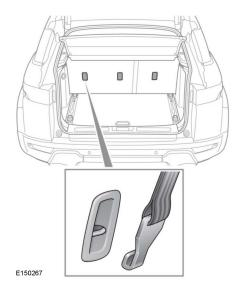
Your vehicle may be equipped with anchorage points on the back of the second row seat frames. These should be used to attach straps from child seats or restraint systems.
