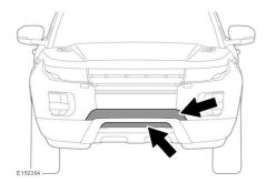
Make sure the areas around air intakes and the front grille are clean and clear of debris. Pay particular attention to the lower grille and radiator. Failure to do so may cause the engine to overheat, leading to severe engine damage.
