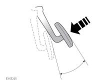
Clutch pedal travel is set at the factory and is non-adjustable.
