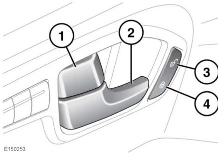
1. Press a locking lever to lock a door. Pull the lever back to unlock. Operating either front door locking levers will lock or unlock all of the doors.
