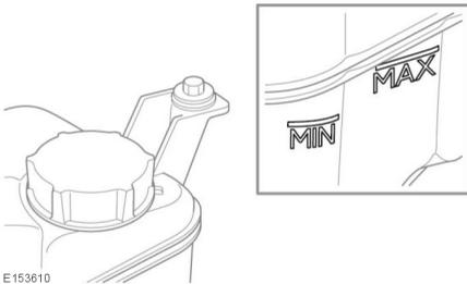
Make sure the coolant level remains between the **MIN** and **MAX** indicator marks on the side of the expansion tank.
