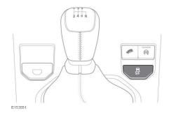
To disable DSC, press and briefly hold the DSC OFF switch. The DSC OFF warning lamp will illuminate. See 92, DYNAMIC STABILITY CONTROL (DSC). Deactivating DSC also reduces the level of Electronic Traction Control (ETC) intervention and may lead to an increase in wheel spin.
