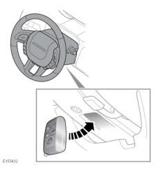
1. Position the Smart key flat against the underside of the steering column with the buttons facing downwards.
