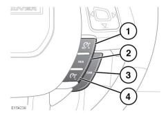
SET+: Press to set the speed or to increase the set speed. The cruise control warning lamp will illuminate to confirm cruise control is operational. See 46, CRUISE CONTROL (GREEN).
