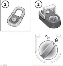
2. Load securing lashing eyes: To assist in safely securing large items of luggage, 4 lashing eyes are located in the rear loadspace floor.
