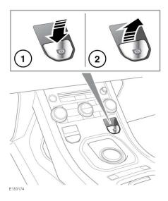
With the ignition turned on, depress the brake pedal, then press down and release the EPB switch. This will release the EPB. 2. With the vehicle stationary, pull up and release the EPB switch. This will apply the EPB. The parking brake warning lamp will illuminate to indicate that the parking brake is applied. See 43, PARKING BRAKE (RED).
