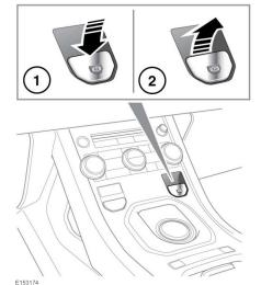
With the ignition turned on, depress the brake pedal, then press down and release the EPB switch. This will release the EPB. 2. With the vehicle stationary, pull up and release the EPB switch. This will apply the EPB. The parking brake warning lamp will illuminate to indicate that the parking brake is applied. See 43, PARKING BRAKE (RED).
