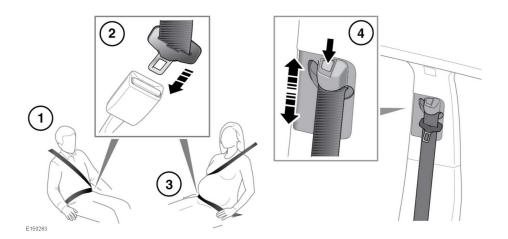
Putting on a seat belt: Draw the belt out smoothly, make sure the belt height, the seat and your position on the seat, are correct.
