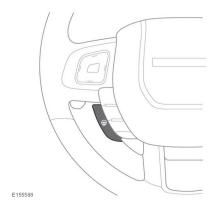
Press to switch on the steering wheel heating. Press again to turn off.
