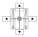
Touch the arrow soft keys to move the sound focal point to the desired area of the vehicle. Alternatively, touch the sound focal point and 'drag' it to the required position.
