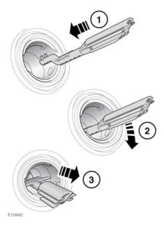
Reset the misfuel protection device as follows:
