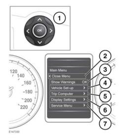
A number of vehicle features and display settings may be configured via the Instrument panel menu.
