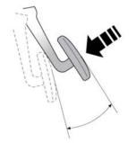
Clutch pedal travel is set at the factory and is non-adjustable.
