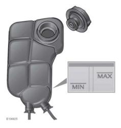
Make sure the coolant level remains between the level indicator marks, located on the side of the expansion tank.
